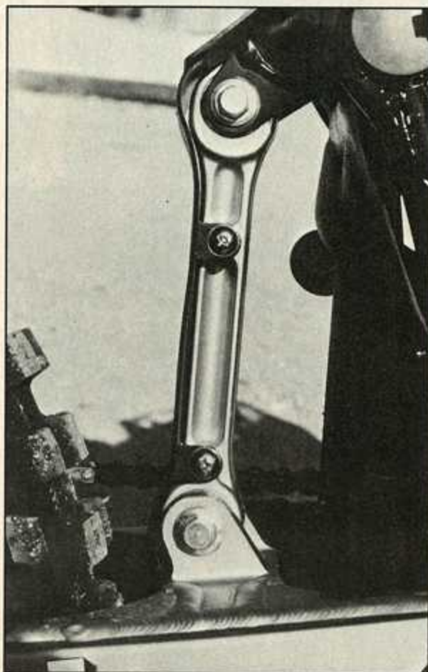
Kawasaki's single dog-bone rear strut is mated to a Kayaba shock. Excellent feel isn't hampered by the lack of adjustability in compression stroke.
