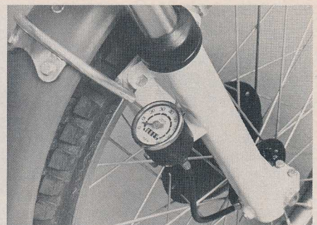
A Marzocchi fork offers six-and-one-half inches of travel. The high-tensile steel fork brace is quite sturdy.
