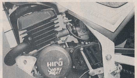
Carburetion is handled by a 27mm Amal. Note the sturdy footpegs and the well-protected chain tensioner.
