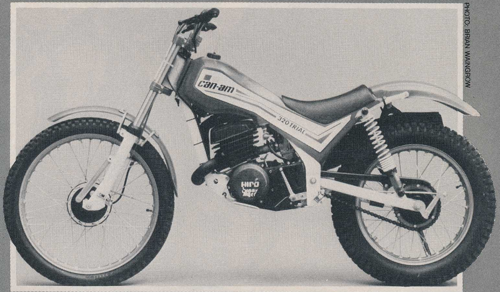
The 320T is nine pounds lighter than the 310T. The aluminum skid plate is rubber padded.
