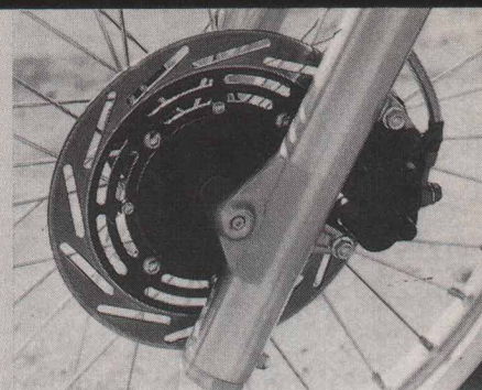
▲ The Honda's front disc brake is slotted to look like the factory bikes.
