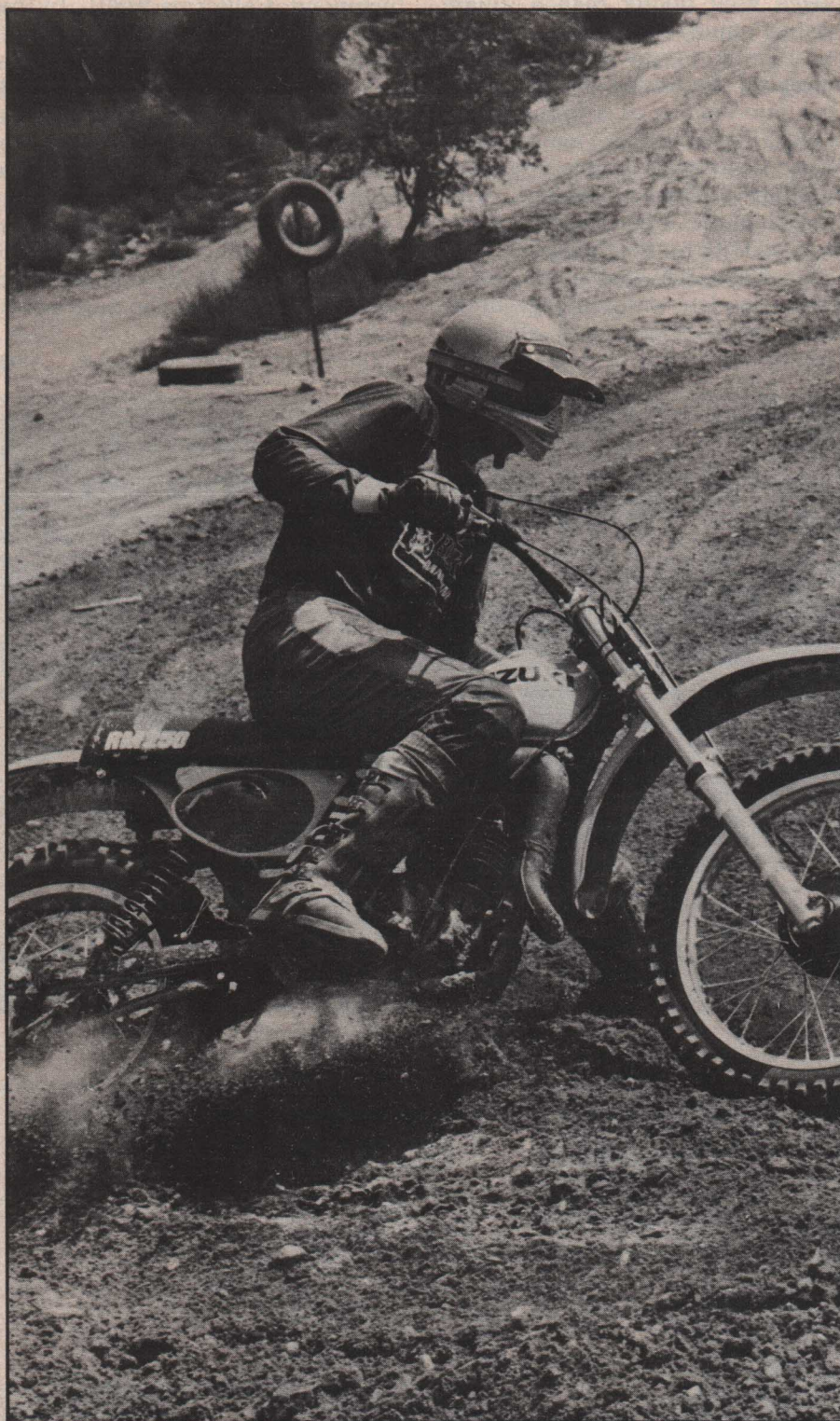
The 1977 long-stroke engine features a redesigned piston, now similar to that found on last year's 370. Porting arrangements are identical to last year's, engine weight is 57.5 pounds.
