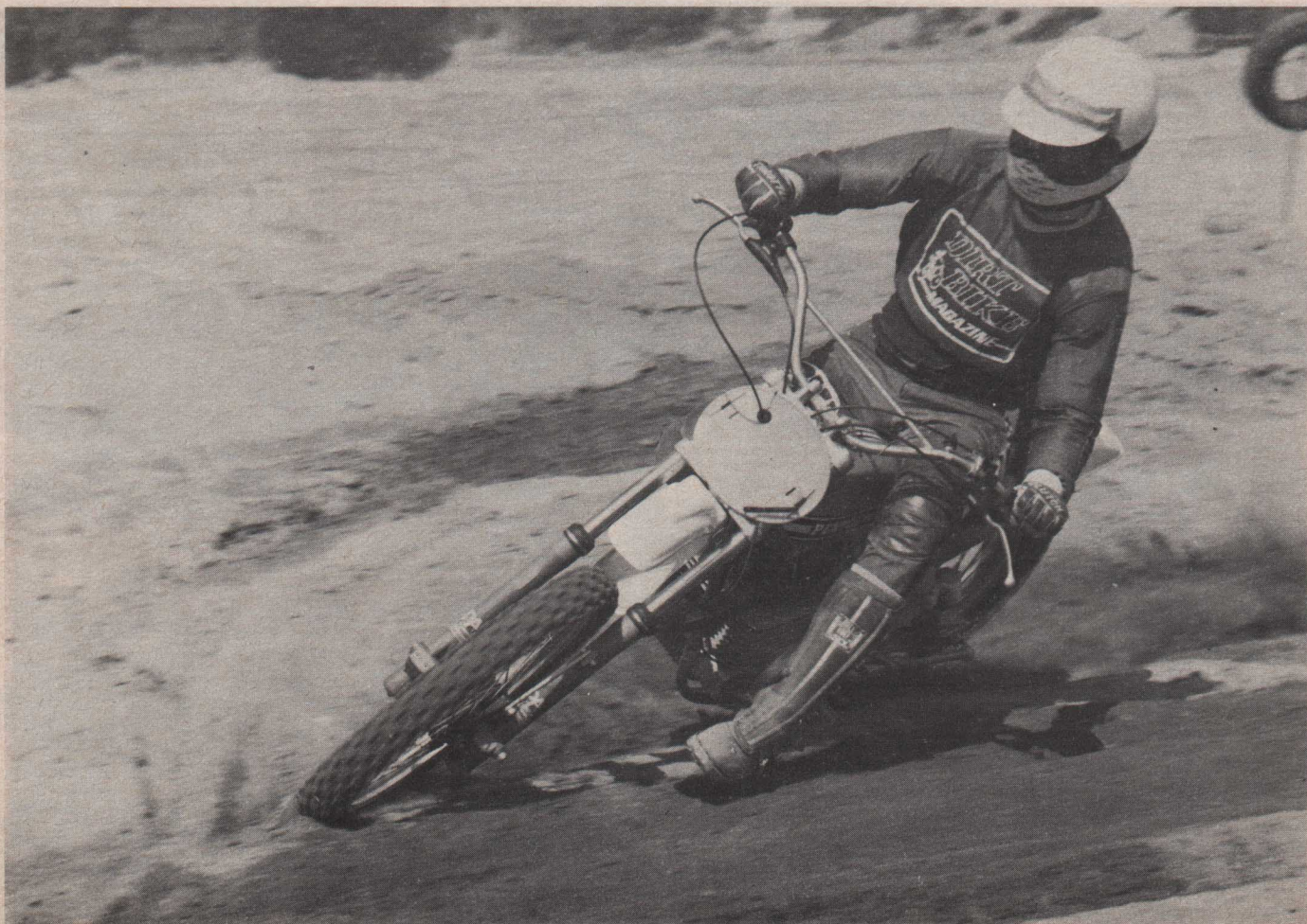
Marzocchi shocks have larger shafts and reservoirs. Chain guide moves up and down.
