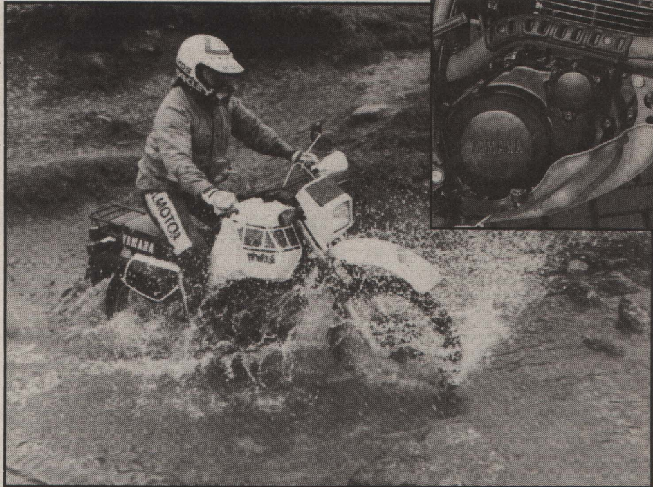
INSET: The 600 Yamaha engine is a slightly de-tuned version of the one fitted to the TT enduro bike.
