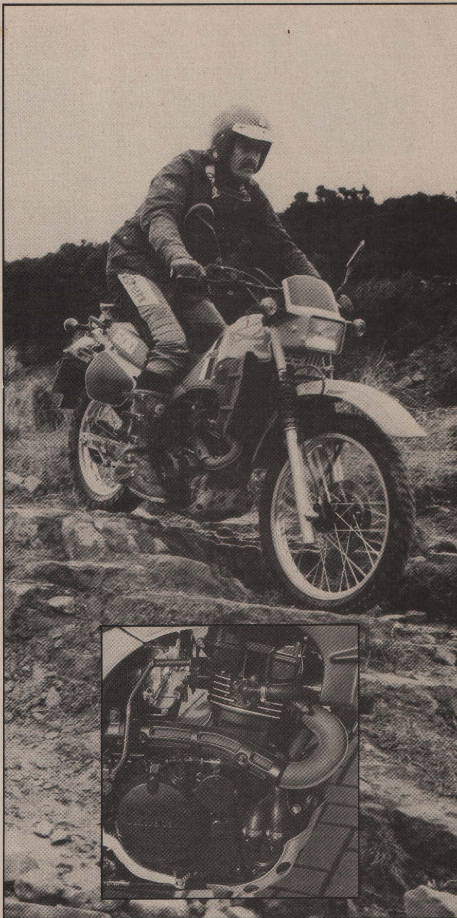
INSET: The liquid-cooled single cylinder engine fitted to the 600 Kawasaki bears a striking likeness to the latest GPz900 roadster.
