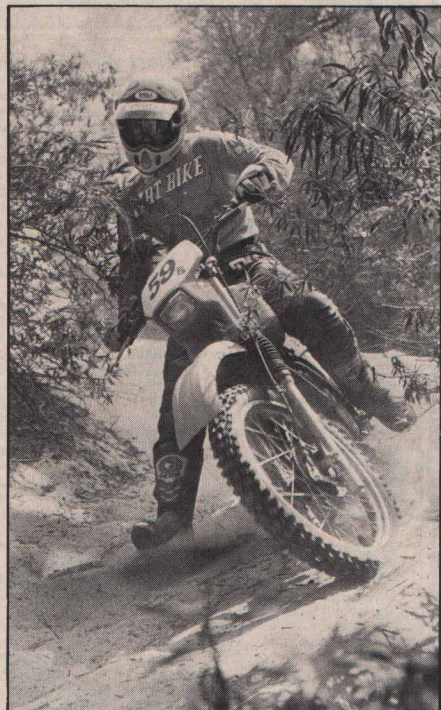
A longish rake on the KDX made it a slow turner, but good all-around power proved to be a blessing.
