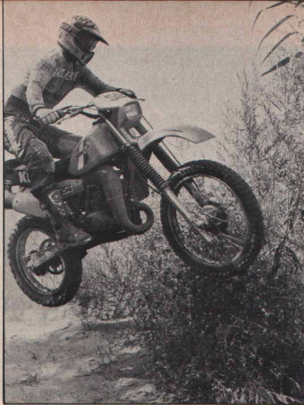
A too soft front end and a dismal front stopper hampered the KDX. Everyone loved the power, its seating and the excellent rear end.
