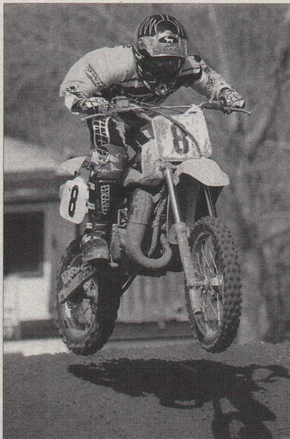
Suzuki needs to bring the RM's chassis up to speed with its engine. The bike's spindly fork and frame are too weak for fast 80 pilots.
