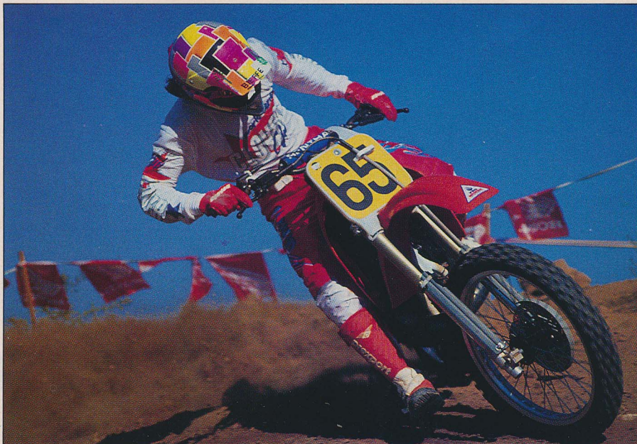
◀ Johnson's bike uses a stock CR500 frame, a Pro Circuit-modified engine and works suspension to do battle with full works GP bikes. Riding it showed that there really is GP-level performance potential in current motocross bikes.
