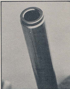
Damper cylinder is retained by rolling over end of fork tube.
