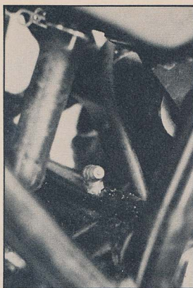
Genuine Zerk fitting on swing-arm pivot fits U.S. grease guns.
