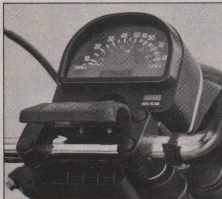
A hinged plastic compartment at the Yamaha's steering head is convenient for storing change for parking or toll roads. Instrumentation consists of a 85 mph speedometer and lights for high beam, neutral and turn signals.
