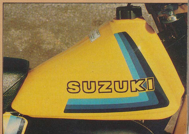
Works style plastic tank holds 2.2 gal. Bars are rear-set and rubber mounted.
