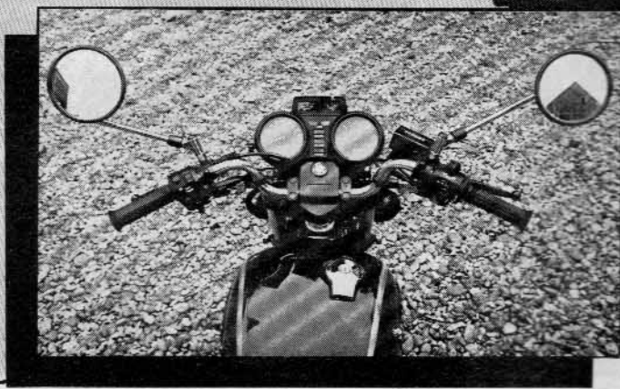
Left: 'bars are just right for boy-racers also in need of a town 'n' touring machine. Ignition lock also incorporates steering lock and there's an additional cable-type anti-theft lock stowed in the seat hump.
