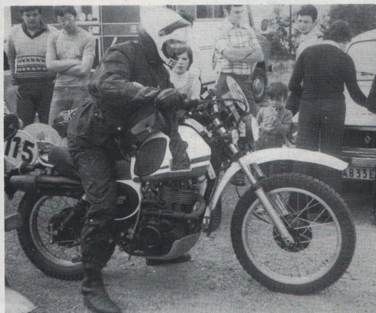
Aime Beche was one of several French riders who chose the Yamaha XT500 single cylinder four-stroke 'thumper' as his mount for the Pyrenees Rally. His is fitted with an extra-large petrol tank.
