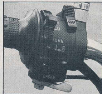
Above: Y'er basic controls don't come any more basic than this on the Kawa with a dipswitch, turn signal switch and horn button next to the clutch lever. Below: Kawasaki has all-enclosed rear chain and non-adjustable suspension units.
