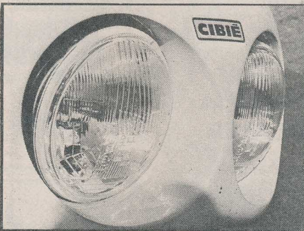
Twin Cibies in the Harris fairing gave the Honda the endurance race look as well as improved night penetration.
