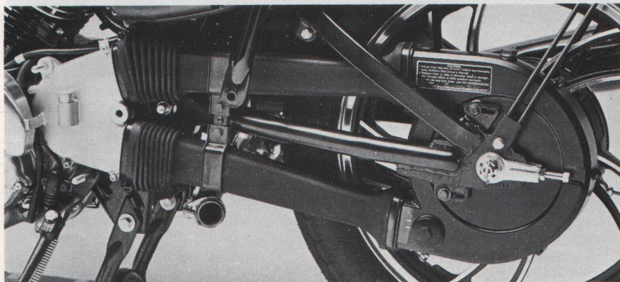
The 920 uses a chain final drive. The chain is fully enclosed and is constantly bathed in a lithium grease.
