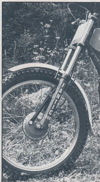
The front end is Marzocchi but Fantic alter the damping.
