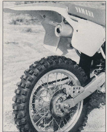
You have to file the WR silencer's rib to fit a spark arrester, and the result is still too loud. Get an Answer Sneaker. The Yamaha rear brake is the strongest of the bunch, but we hate the tire.
