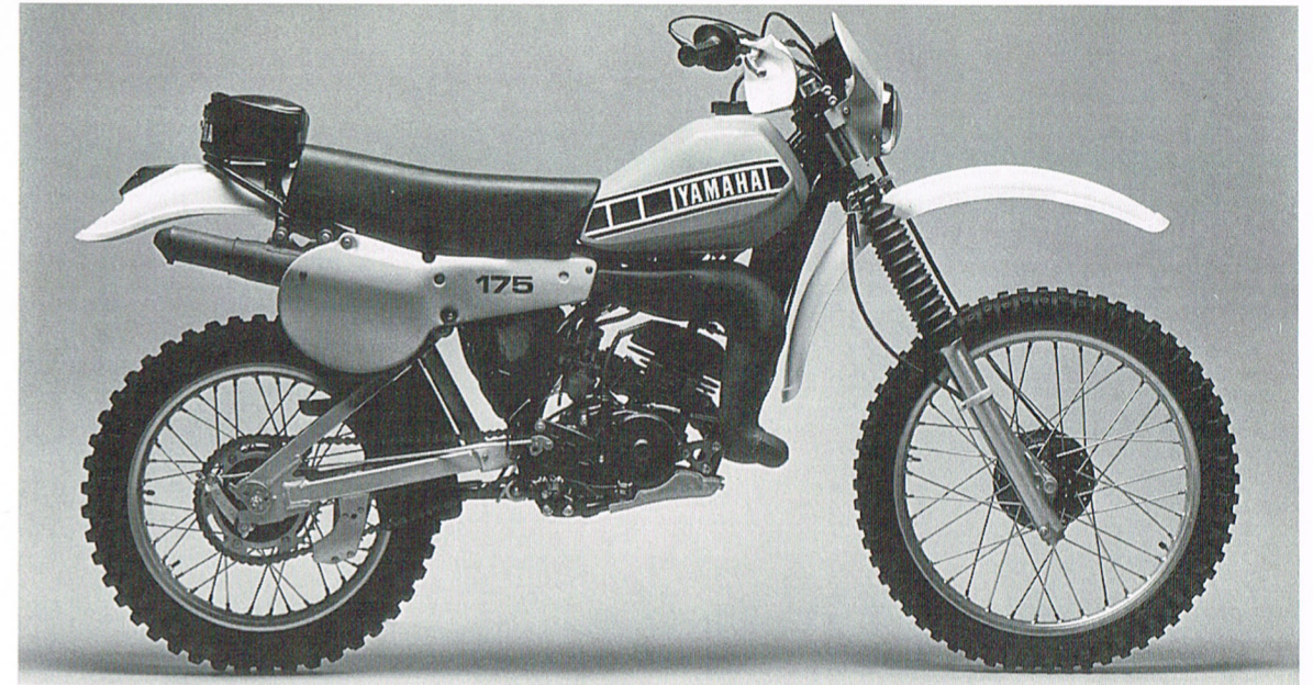
Above For 1980, the IT175 received the same chassis upgrade as was applied to the YZ models that year
