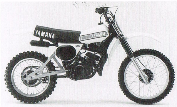
Above Most striking change to the YZ series for 1978 was the use of an aluminium swinging-arm, illustrated here on the 125
