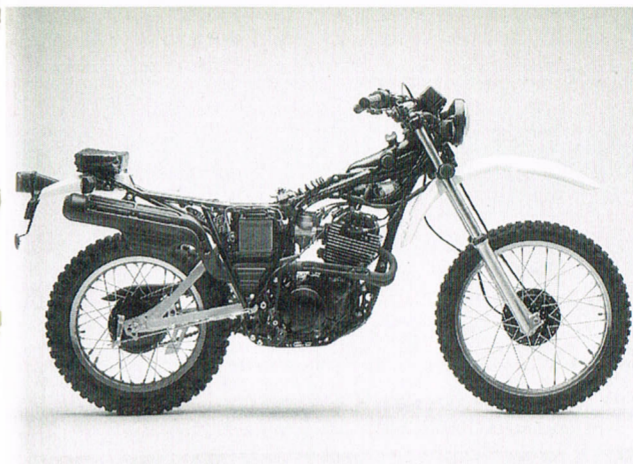
Monoshock suspension and an aluminium swinging-arm improved the XT550 enormously but it was not enough to put it back at the top of the tree
